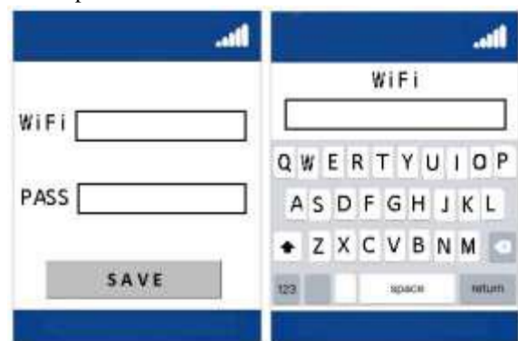
Fig. 4. The main screen for entry login acces and password, created with ITEAD editor for Nextion display.
